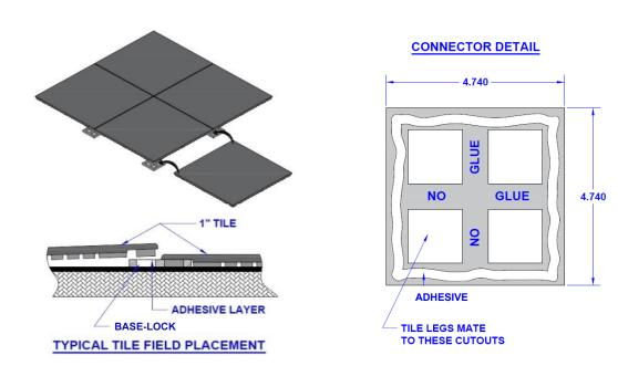
Note: Adhesive spills must be removed <u>while still wet</u>. Use a dry rag to pick up the majority of the adhesive. Wipe the remaining residue with a rag dampened with mineral spirits. Cured adhesive can only be removed from surfaces by mechanical means, such as scraping or sanding.
