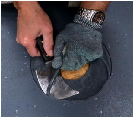
Using an angled skiving knife
