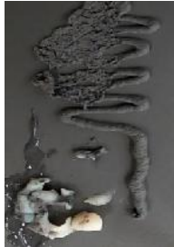
Incorrect: Cold Rapid Weld
